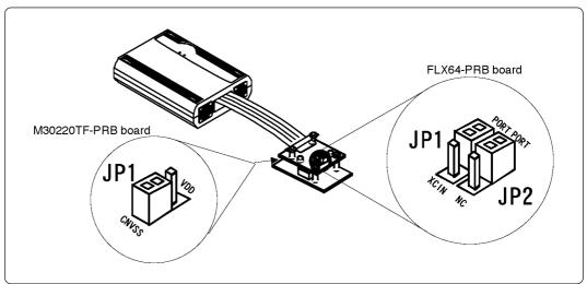
Figure 3.1 Positions of the switches and their factory-settings
